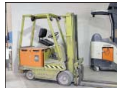
Clark Electric Lift Truck, #EC500-55F S/N E355 277 3505FA, Closed Mast 82", Max Lift 185", 48" Forks
